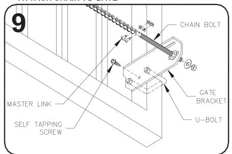
• Attach the gate bracket to the gate as shown using the round or square u-bolts for round or square gate frames respectively. Attach the chain to the gate brackets using the chain bolt and master link as shown. If necessary, the chain may be easily shortened using a chain breaker. Adjust the height of the gate brackets until the chain is level and firmly tighten the u-bolts. For round gate frames it may be necessary to drive the self tapping screw through the gate bracket, and into the gate.
